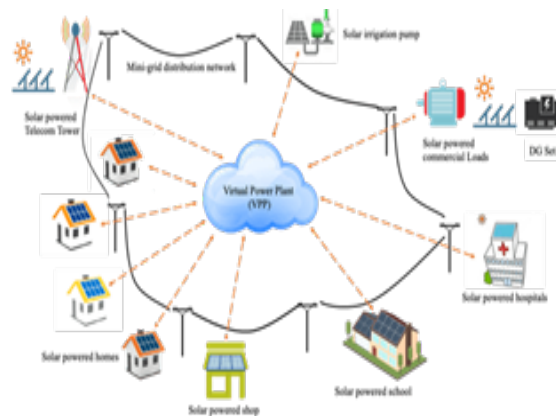
Figure 2: Conceptual diagram of a mini-grid with distributed PV & Battery systems operated under a virtual power plant
