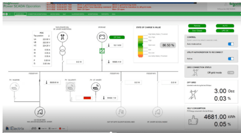
Fig.5 Main screen of the SCADA system during the islanding test on November 2022.
