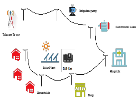
Figure 1: Conceptual layout of a solar PV-based mini-grid project with different loads
