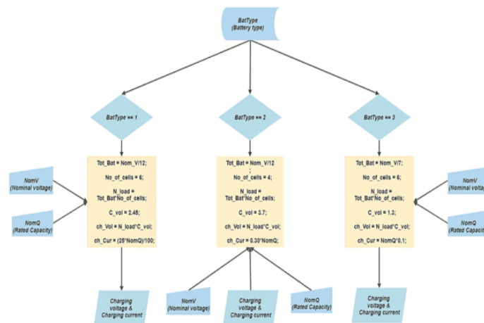
Fig 4. Algorithm for identification of Charger Control parameters
